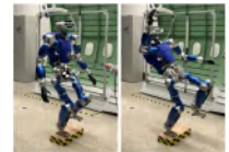
TORO generating centroidal angular momentum after being pushed.
