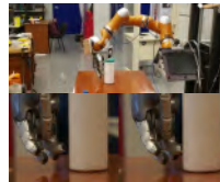
Experimental set up. Our robot pushing a cylinder.
