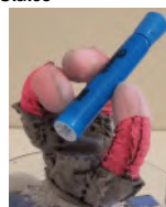
CMU Foam Hand III performing an in-hand manipulation.
